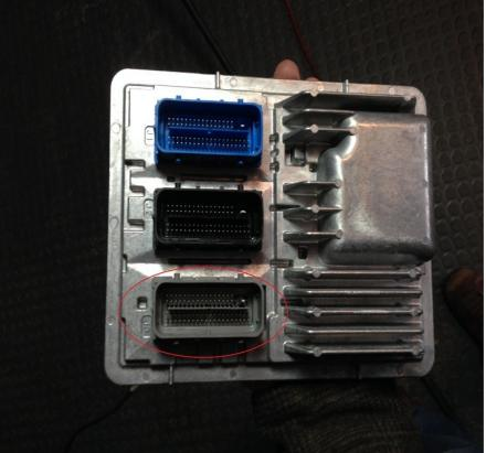
You will need to open the haness to insert the new pin (molex mx64 femal) into position #70 as shown:
