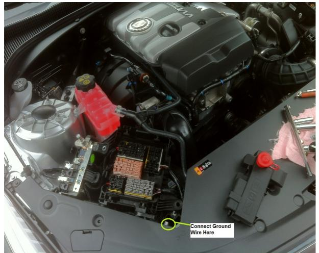
You can remove the engine electrical center as shown above to allow easier access to the ECM harness, but it is not necessary.
