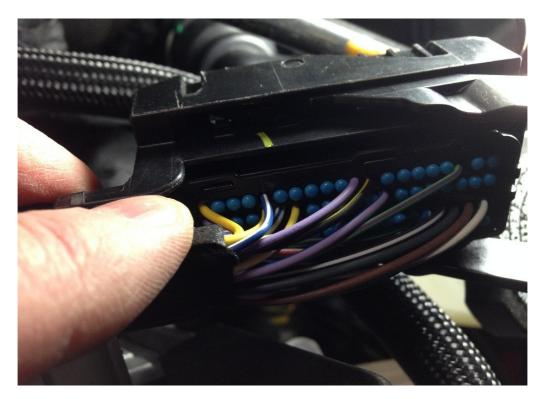
Once the connectoris open you can remove the blue plug at position #70 and insert the new wired pin:
