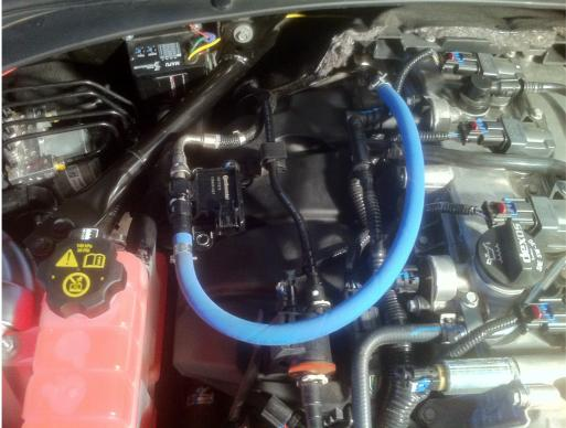
The signal wire from the flex fuel sensor will be connected to ECM harness X3 (Grey) pin #70. The +12V power can be pulled from any switched relay – I suggest taping fuse #48 (Insturment Panel Body Ignition) or #49 (Fuel System Control Mondule / Ignition) in the engine bay electrical center and connecting the ground to the post near the electrical center:
