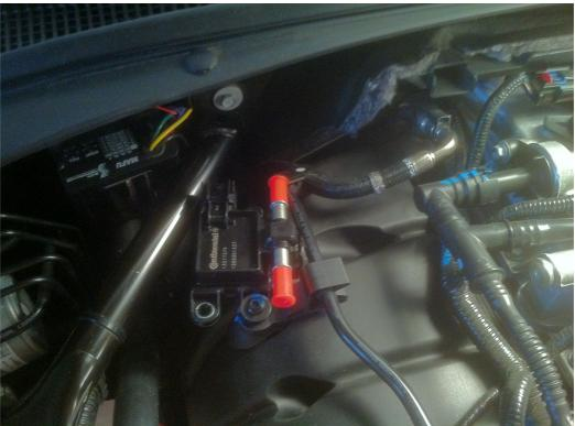
2) Pull Fuse #37 from the rear fuse compartment to de-energize the low pressure fuel pump.
