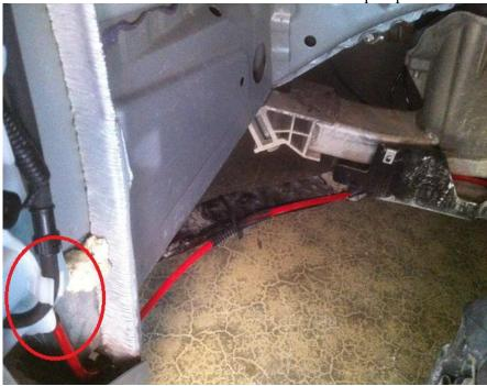
Connect the wiring (connect the green/white wire from the mass air flow sensor to the mass airflow signal wire on the controller):
