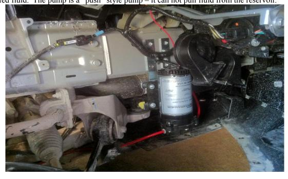
Tap the windshield washer reservoir and connect the reservoir to the pump:
