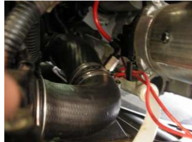
Nozzle mounted in charge pipe.
