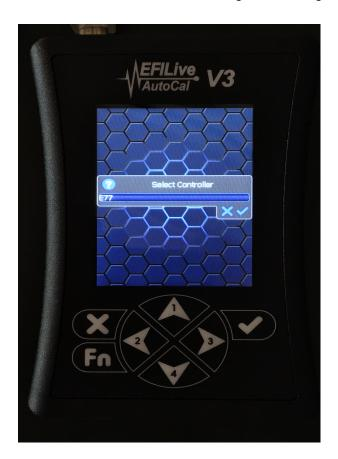
The display will show a progress bar and will prompt you to turn the key to the "Off" position when it is finished. Press the ✓ again and it will run a count-down timer to allow the computer in the car to reset before you start the engine.
