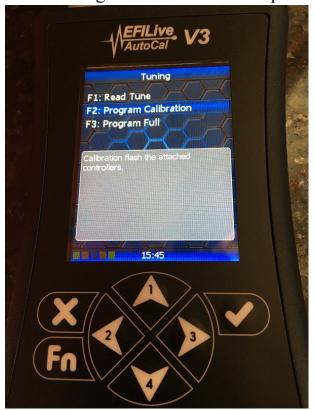
Your installed calibrations will be listed: Select the file you wish to install, turn the key on the car to the ON position but do not start the engine, then press the ✓ button to begin the flash.
