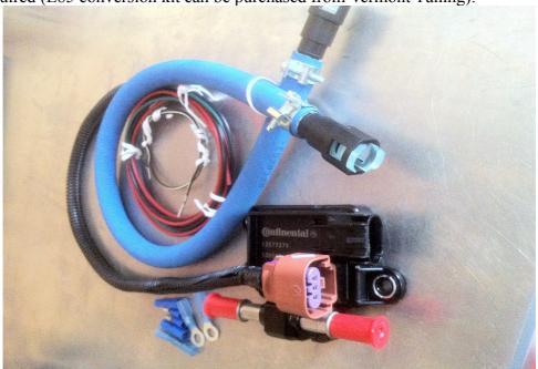
Ethanol sensor Ethanol sensor harness/pigtail Female molex mx64 pin 12" flex fuel hose GM style fuel quick connectors ATR MICRO2 Fuse tap (not supplied)
