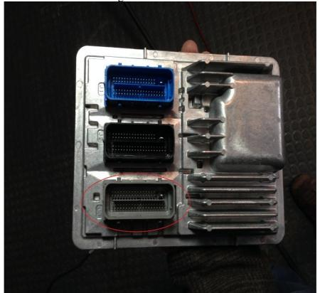
You will need to open the haness to insert the new pin (molex mx64 femal) into position #70 as shown:
