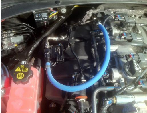
The signal wire from the flex fuel sensor will be connected to ECM harness X3 (Grey) pin #70. The +12V power can be pulled from any switched relay – I suggest taping fuse #42 (Insturment Panel Body Ignition) in the engine bay electrical center and connecting the ground to the post near the electrical center:
