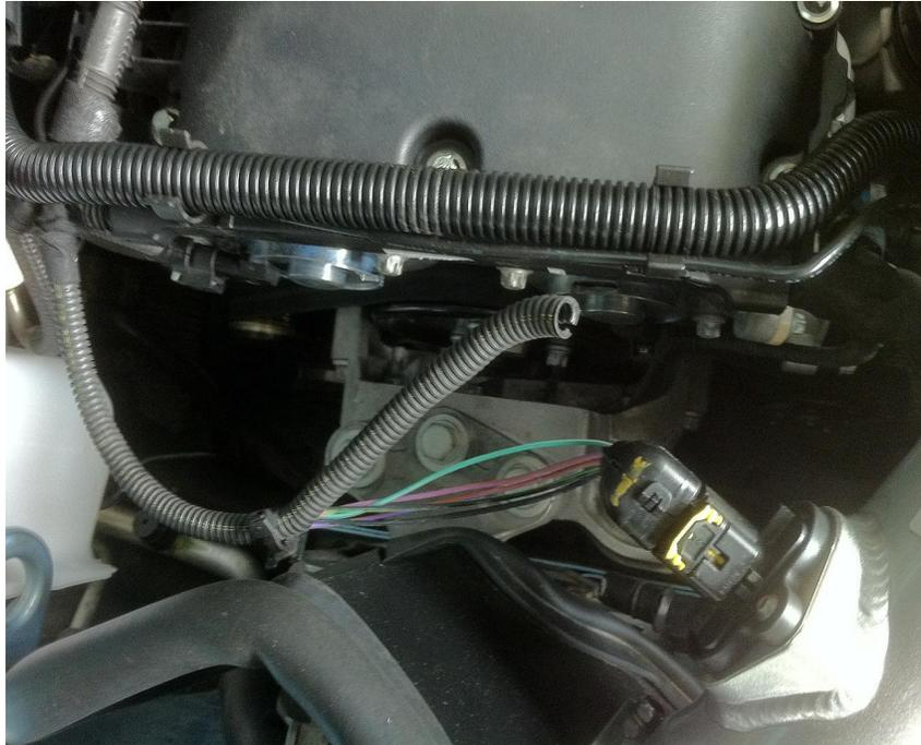
Tap the intake pipe and install the injector nozzle holder, #2 nozzle, and connect to the pump:
