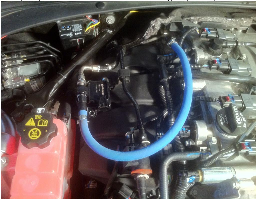
The signal wire from the flex fuel sensor will be connected to ECM harness X3 (Grey) pin #70. The +12V power can be pulled from any switched relay – I suggest taping fuse #48 (Instrument Panel Body Ignition) or #49 (Fuel System Control Module / Ignition) in the engine bay electrical center and connecting the ground to the post near the electrical center:
