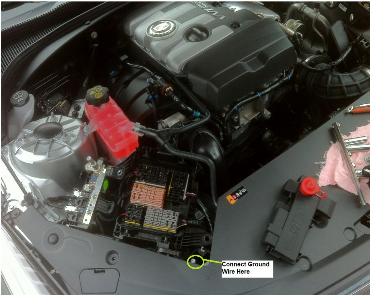
You can remove the engine electrical center as shown above to allow easier access to the ECM harness, but it is not necessary.
