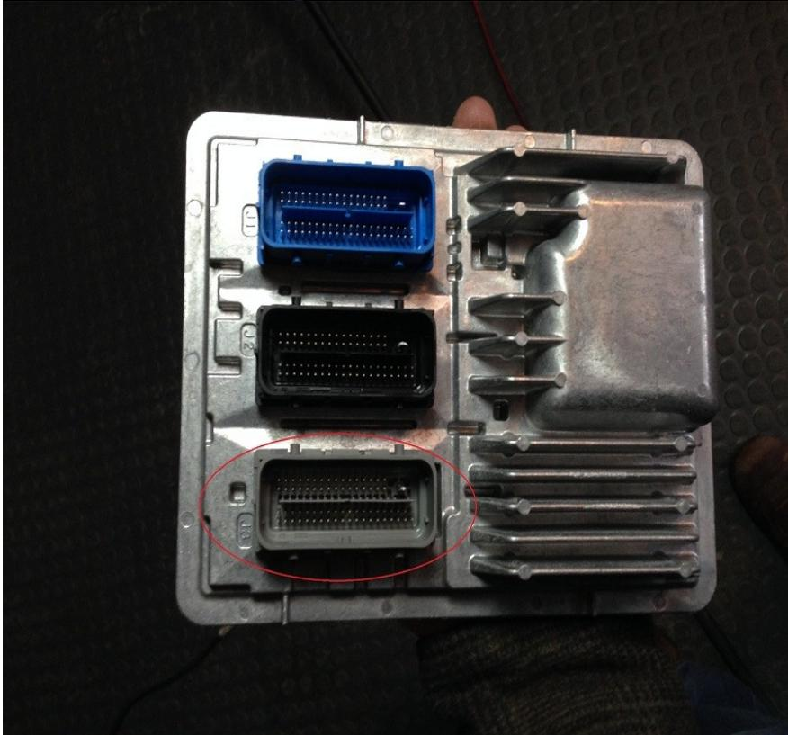
You will need to open the harness to insert the new pin (molex mx64 femal) into position #70 as shown:
