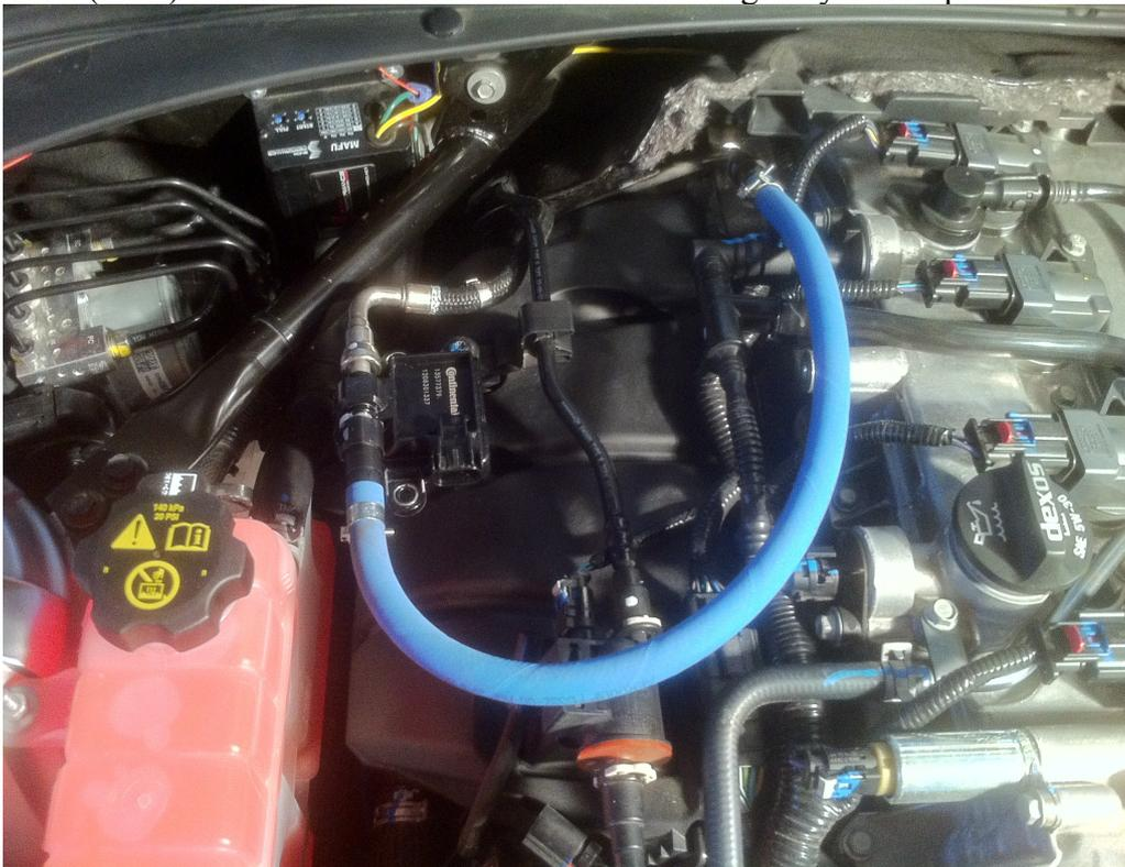
The signal wire from the flex fuel sensor will be connected to ECM harness X3 (Grey) pin #70. The +12V power can be pulled from any switched relay – I suggest taping fuse #42 (Instrument Panel Body Ignition) in the engine bay electrical center and connecting the ground to the post near the electrical center:
